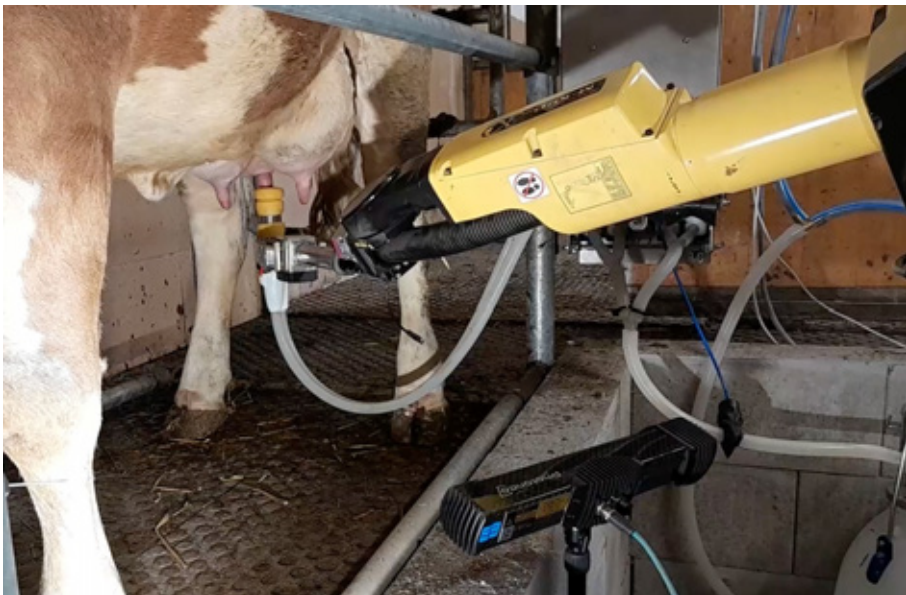
Figure 1. Robotic arm for milking of the cow (internal documents of the company).
