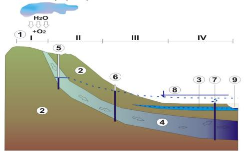
Legend: I Recharge zone, II Zone of good quality of groundwater, III Transitional zone, IV Zone of groundwater with higher content of iron and sometimes manganese, 1 - Infiltration area, 2 - aquitard, 3 - Unconfined aquifer, 4 Confined aquifer, 5 Water well, 6 Nonflowing artesian well, 7 Flowing artesian well, 8 Water table, 9 River.
