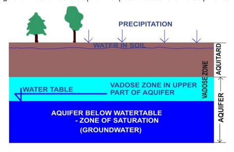
If the saturation zone in direct contact with aquitard in overlie of the aquifer, with marked inter-granular type of porosity, i.e. if the aquifer is sub-artesian or artesian (Figure 2), due to biochemical processes, anaerobic conditions are created which generates an increased content of iron and manganese in groundwater.
