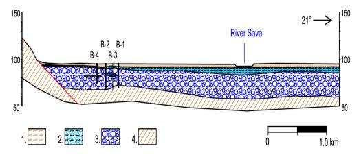
Legend: 1. Clay, 2. Clay and sand with clay below the water table (zone of saturation), 3. Sandy gravel, 4. Underlie aquifer
