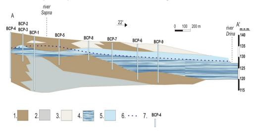
Legend: 1. Clay, 2. Marl, 3. Sand and sand with clay, 4. Aquifer below the water table, 5. Vadose zone of aquifer, 6. The water table, 7. Borehole
